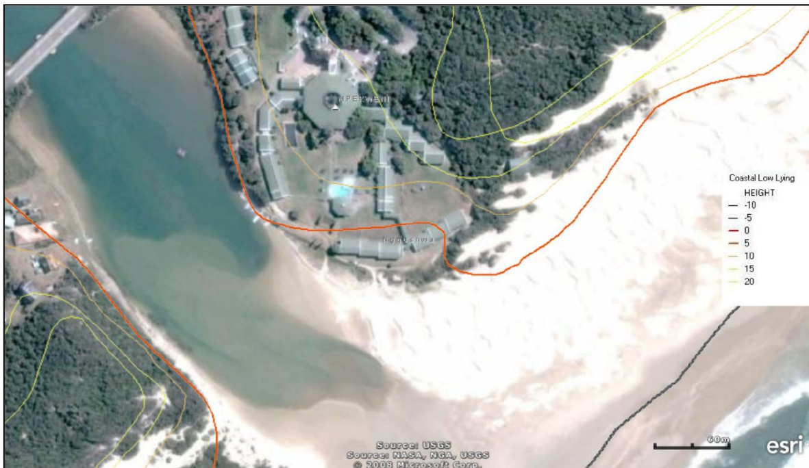
Figure 13: Coastal infrastructure Mpekweni that lies below the 5 metre contour, thus vulnerable to sea level rise.
