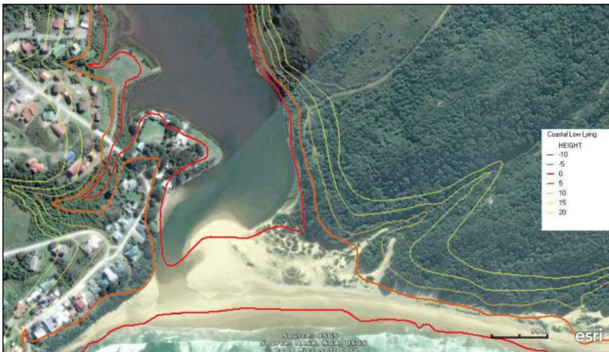
Figure 14: Coastal infrastructure at Morgan Bay that lies below the 5 metre contour, thus vulnerable to sea level rise.
